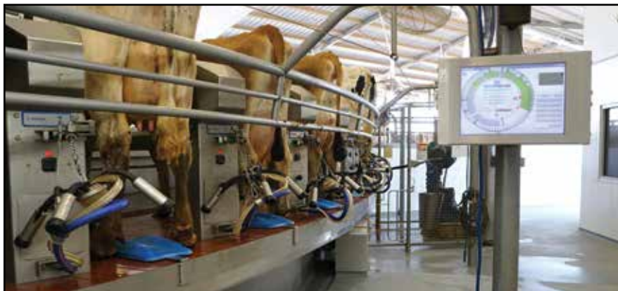
Cows at Vierra Dairy are milked in a state-of-the-art parallel rotary parlor, fitted with blue cow guards that ideally position feet for milking and an interactive data display that keeps workers abreast of activities in real time.
